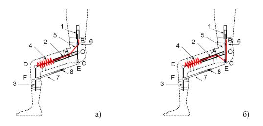
Figure 2. Walking and sitting assistive devices with a regulating slider: a - in walking mode; b - in sitting mode.
