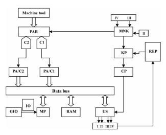
Fig. 4. Diagram of controlling system of elastic-deformable state basing on microprocessor
