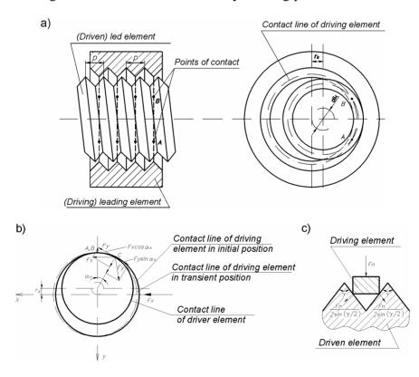
Fig. 2. Computational diagram of vibratory walking pneumatic drive: geometry of driving and driven elements' co-operation – a; scheme of driving and driven elements' contact – b; scheme of applying the component of force on the side of the drive
