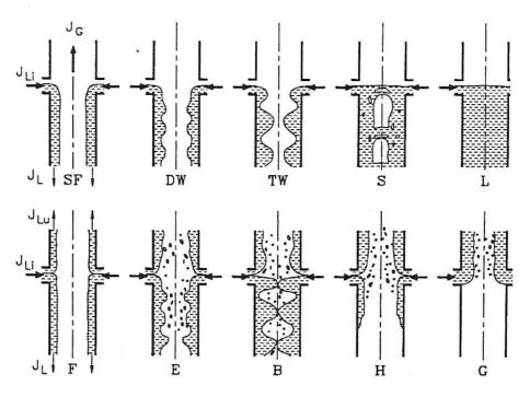
Fig. 2. Flow structure in counter – current flow
