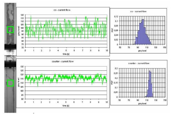
Fig. 3. Flow structure: foam in co – current flow and liquid downflow in counter – current flow
