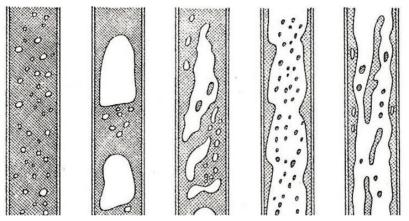
Fig.1. Flow structure in co - current flow: a). bubbly; b). lock; c). foam; d). ring; d). dispersed
