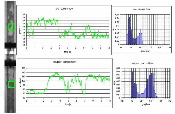
Fig. 4. Flow structure: lock in co - current and counter - current flow
