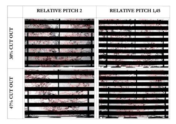
Fig.1. Exemplary velocity vectors for the two-phase flow in the channel with five baffles and 30% cut out with two different relative pitches
