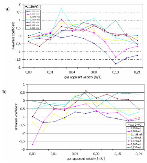
Fig.2. Distribution of skewness coefficient: a) t/d = 2; b) t/d=1,45
