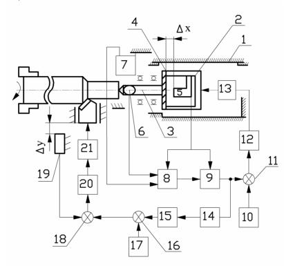
Fig.1. Functional outline of the mechanical processing accuracy controlling system
