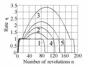
Fig. 2. Dependence of rate  $\eta$  on diameter and run out of the blank: 1 - 3 - diameter o20, 4, 5- diameter o30; run out (mm): 1- 0.1, 2- 0.15, 3 - 0.2, 4 - 0.2, 5 - 0.25
