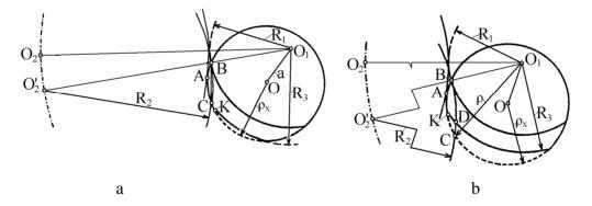
Fig. 1. Schemes of cutting of a wheel into the blank: a – at contact point B wheel cuts only sector BAC; b – wheel cuts sector BAKD
