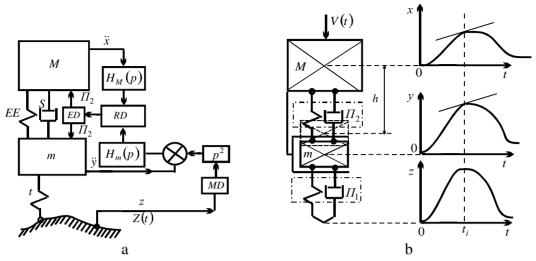
Fig. 1. The scheme of an active suspension of the vehicle (a) and classical two mass system with the limited general movement of a suspension (b):
